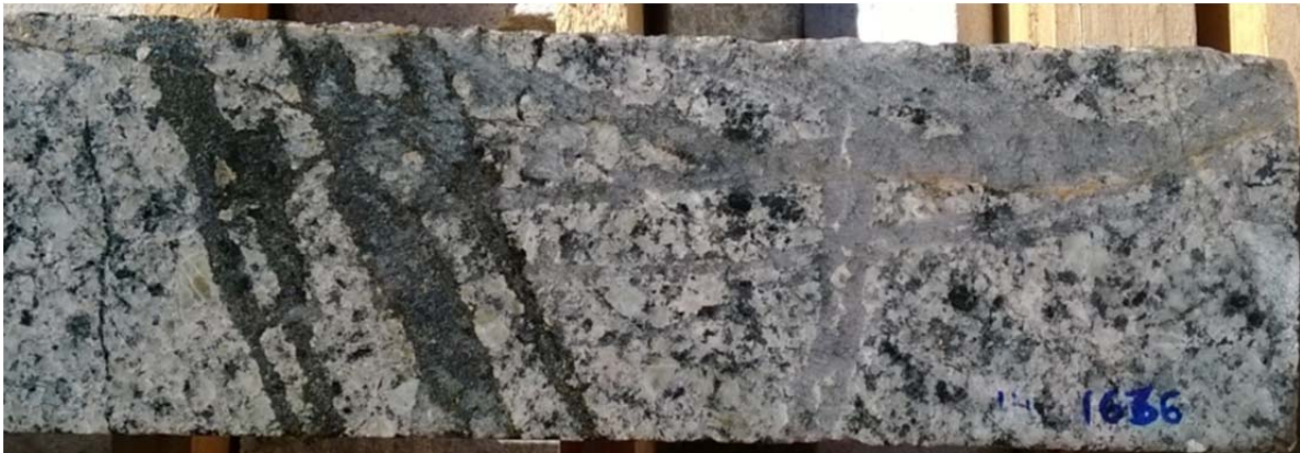
Figure 7.5 VALDD13-014, 1634-1636 m - 0.8 ppm Au, 1.5% Cu. Valeriano granodiorite with K-feldspar and biotite potassic alteration cut by early-biotite and A-type quartz vein stockwork with chalcopyrite and bornite mineralization.
