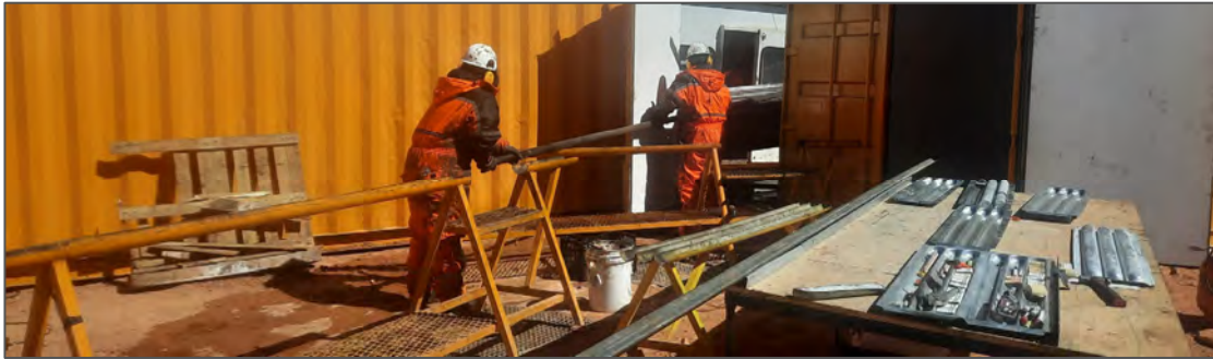
Figure 11-6: Recovery of drill core from drill hole ATXD24 as witnessed by the QP.
