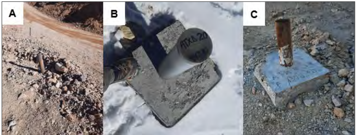
Figure 11-7: Photographs of collar monuments for three holes at Valeriano, Hochschild A, ATEX B-C.
